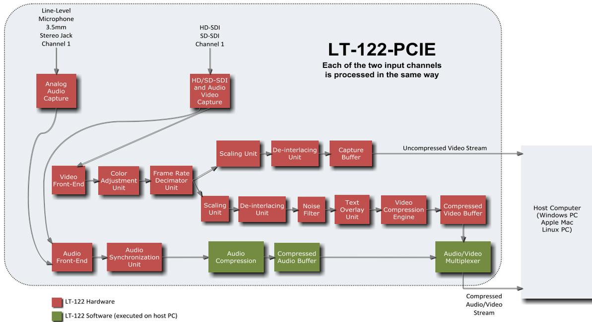
The LT-102-PCIE is comprised of several functional elements. Their operation as well as their function is described in this section. The diagram above shows the various elements and their interconnections. Note that only one of the two acquisition/compression channels is depicted.
