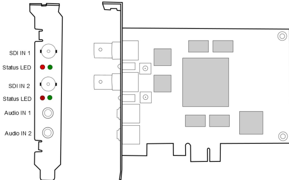
The bracket on the left shows the connector configuration
